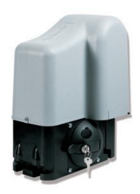
Anti-crush safety is ensured by an adjustable twindisc clutch which reduces the thrust force of the gate in case of an obstacle.
